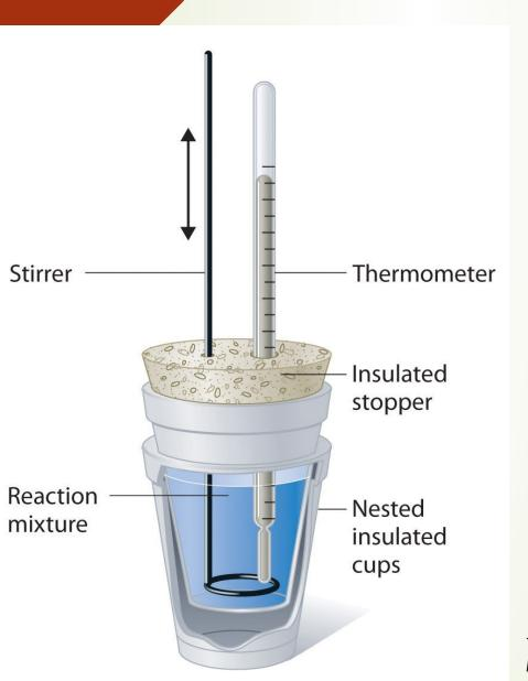
Measuring heat transfers during a chemical reaction (e.g., coffee cup calorimeter)
