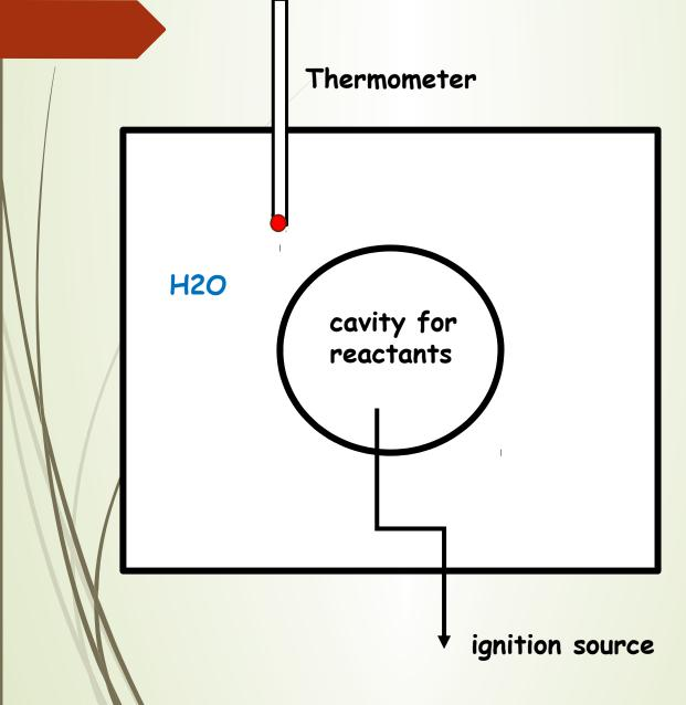
Bomb calorimeters are used in reactions where one or more of the reactants is a gas. The "bomb" is made of rigid materials, such as steel, and includes a cavity (for reactants) surrounded by a water bath.
